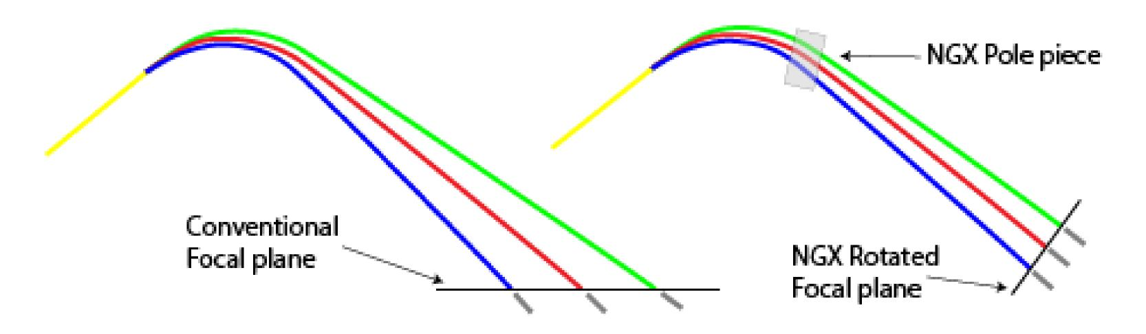
Figure 2. NGX pole piece rotates the image focal plane improving collector efficiency and lowering the collector volume.
