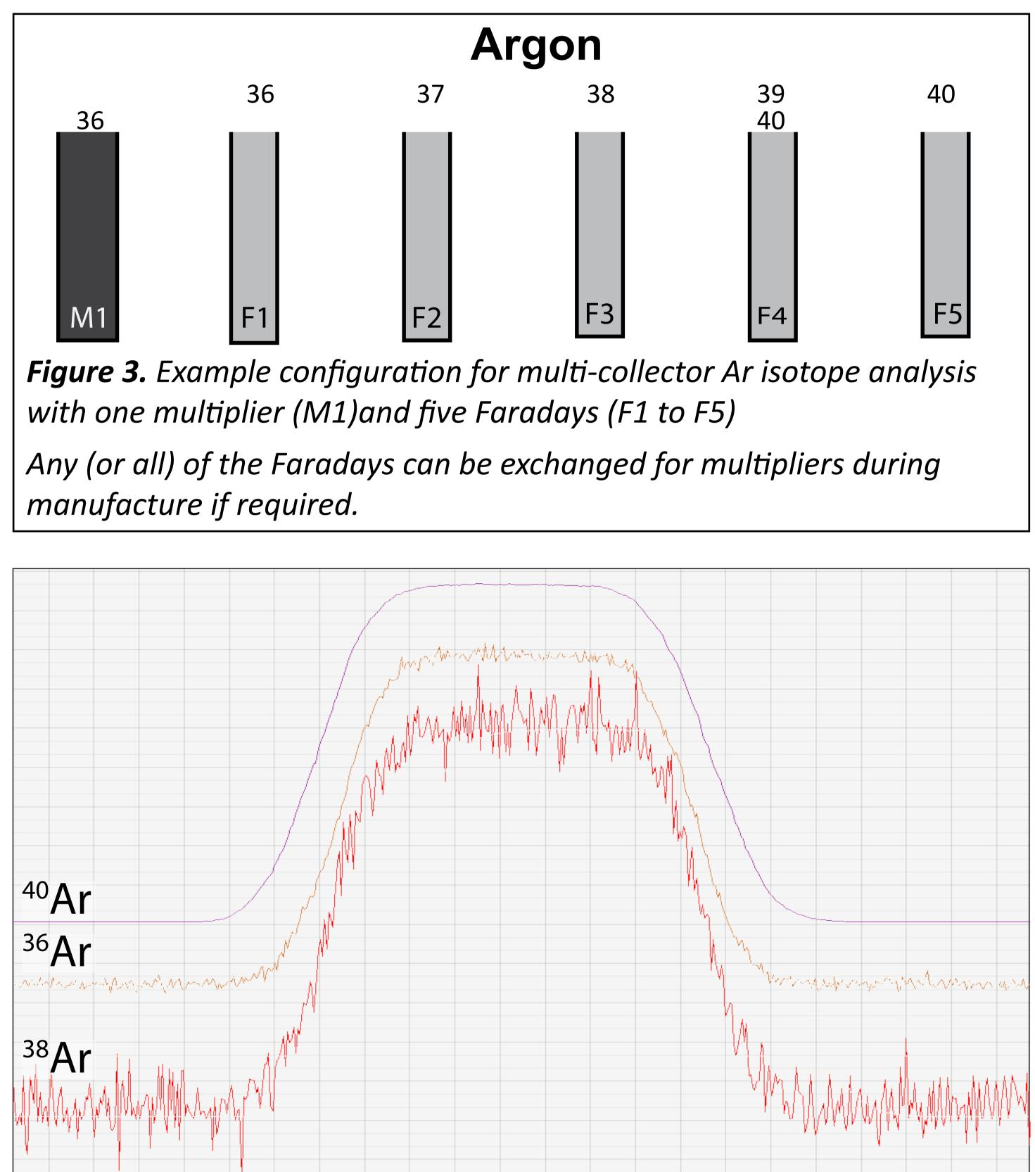
**Figure 4.** Coincidence of <sup>36</sup>Ar, <sup>38</sup>Ar and <sup>40</sup>Ar. Each trace is automatically scaled.
