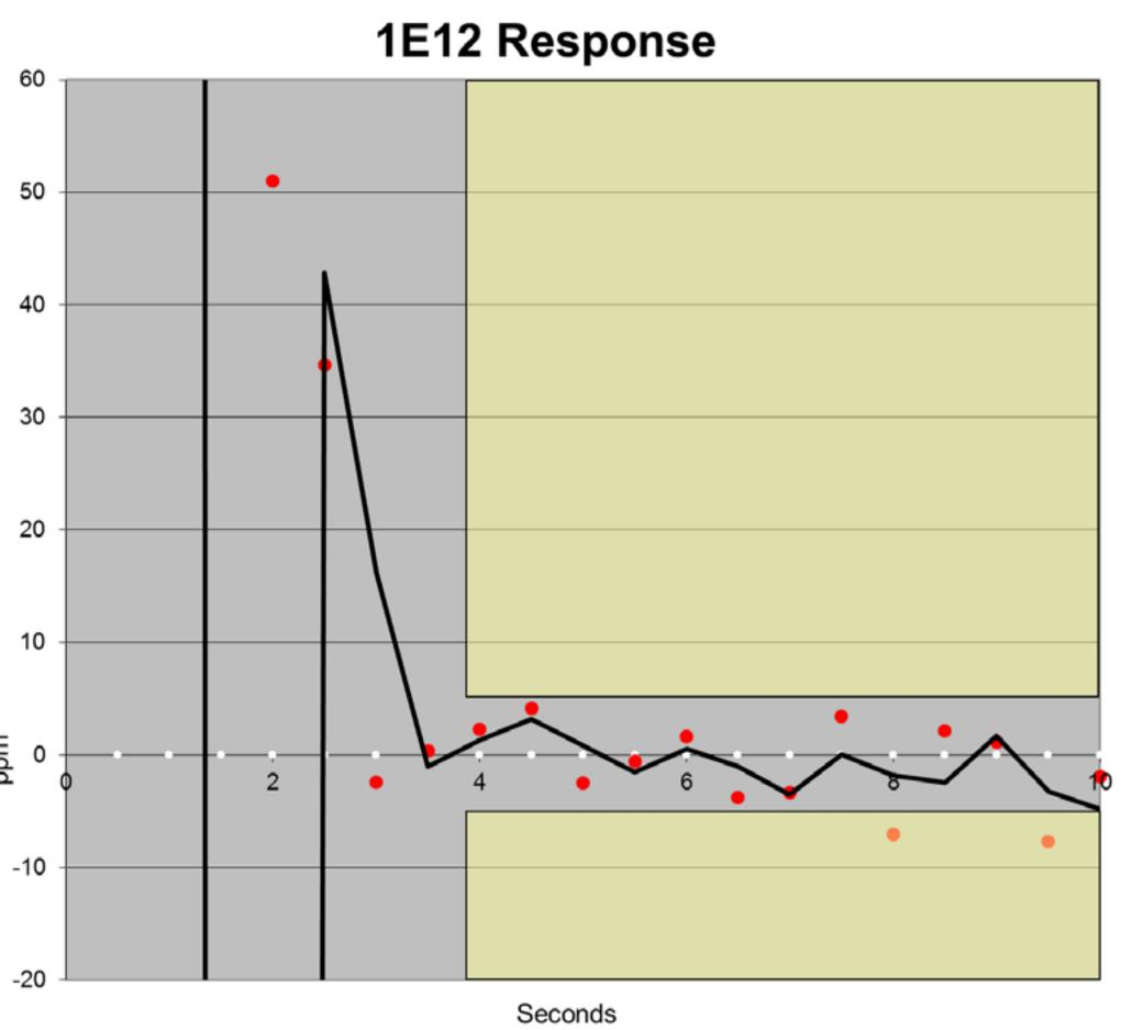
**Figure 6.** Response of NGX  $1e^{12}\Omega$  Faraday amplifiers in the 10 seconds after a 5 volt/5e<sup>-12</sup>A ion beam was switched off the Faraday.
